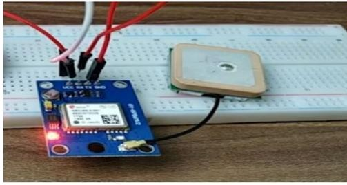
Fig 6 . Module GPS Testing
