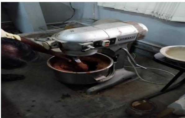
Figure 4. Preparation of clay layer
